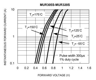
**Fig.6 Typical Forward Characteristics**
