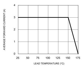
Fig.1 Forward Current Derating Curve
